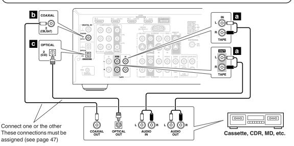
• To connect the recorder digitally for playback, use connections **a** and **b**, or **a** and **c**.
